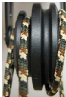
Example 2 of incorrect alignment.
