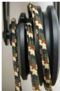
Example 1 of incorrect alignment.
